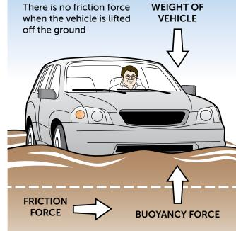
The vehicle will be carried when BUOYANCY FORCE is greater than VEHICLE WEIGHT.
